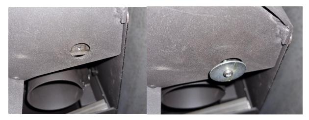
**Step 4.** Align the hole of the raised part of the U-Profile with the corresponding hole in the bottom plate. Then place the outer ears of the front plate underneath each of the U-Profiles raised bits. Insert the screw and screw the parts together:
