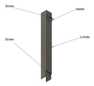
The brace will be fitted using some of the existing holes in the bottom plate of the stove:
