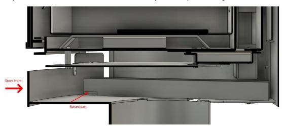
**Step 3.** Align the hole in the back of the U-Profile with the large hole in the back of the bottom plate, then screw in the screw with a washer on:
