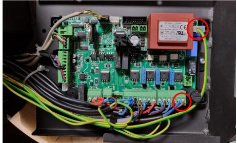
7. Check the fuse to see if this is blown. The fuse is accessed by unscrewing the cap on the black tube on the control board:
