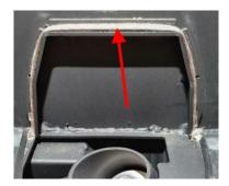
Remove the gasket guide and remount the brazier and vermiculite.
