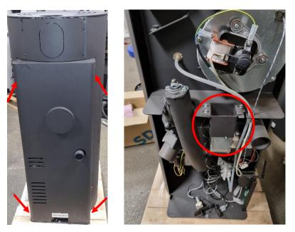
2. Disconnect the two cables to the fan:
