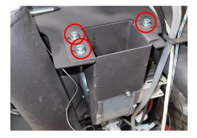
4. Now remove the four screws which attaches the bracket to the fan:
