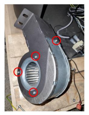
5. Before mounting the bracket to the new fan, make sure that the holes in the fan's air duct align with the holes in the fan's cover plate. The cover plate can be rotated:
