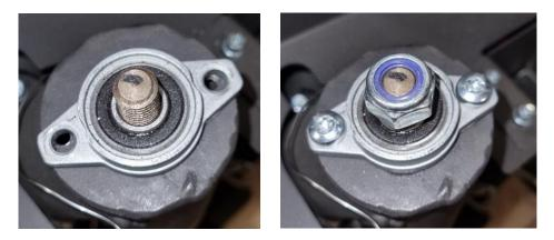
9. To mount the motor to the stove, the motor must be placed correctly: As the axle is not centered on the motor, the short side is placed downwards:
