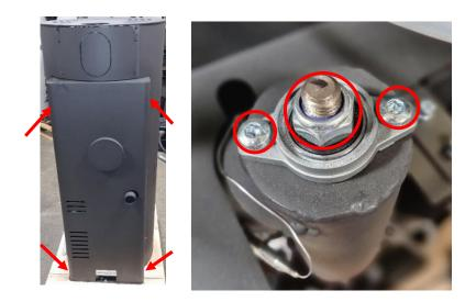
3. Now, unscrew the four screws that mounts the motor to the stove chassis:
