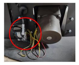
2. Unscrew the four screws on the stove's backplate and remove the backplate. Then remove the nut from the external auger thread, unscrew the two screws in the sides and remove the bearing:
