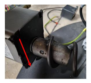
10. Rotate the motor (the round piece) to place the cables to the left so they can easily be connected to the terminal. Screw the motor back into the stove chassis with the four screws. Then you can tighten the nut on the threaded rod on the backside of the stove.
