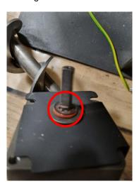
8. Place the pinion screw so it aligns with the flat surface of the motor axle and tighten the pinion screw with the Allen key:
