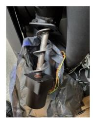
5. Then separate the auger from the motor by unscrewing the pinion screw with a 3 mm Allen key:
