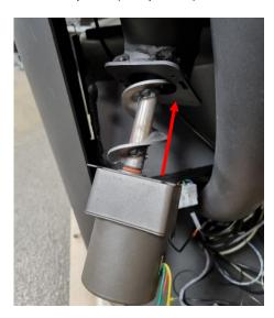
10. Reconnect the motor cables to the terminal as shown below:
