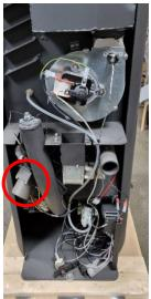
2. Disconnect the motor cables from the white terminal: Press and hold the locking buttons on the terminal, then gently pull the cables out:
