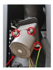
4. Before removing the motor and auger, place a bag underneath to catch the pellets that will fall out of the auger. Then gently pull out the motor and auger – it's easiest if you twist it a little from side to side while pulling.
