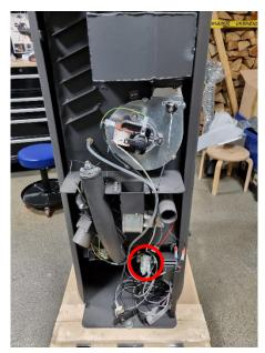
2. Remove the rubber tube from the pressure switch:
