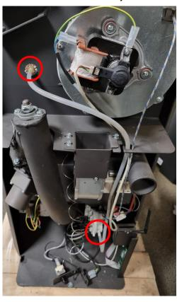
2. Check that the power switches are connected to the right inputs on the pressure switch. Also make sure that they are connected to the control board:
