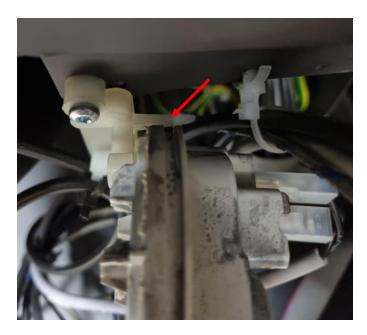
4. Remove the cable connectors from the pressure switch pins:
