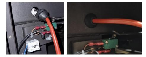
4. The ceramic ignitor can be aligned to the hole, by using a tiny round object that can be inserted into the hole and guide the ceramic ignitor into the right place:
