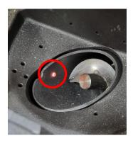
If the ceramic ignitor is not warming up, it is most likely faulty and needs to be replaced.
