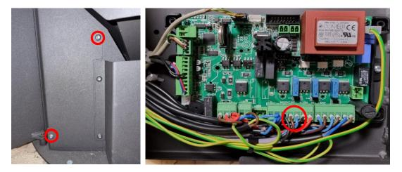
• If this doesn't solve the problem, try exchanging the power socket and cables, and lastly try to change the control board.
