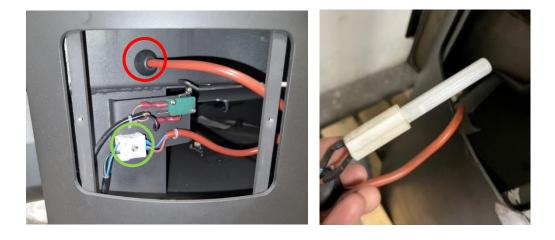
3. Install the new ceramic ignitor. The ceramic ignitor is inserted into a small pipe inside the hole. Mount the rubber sealing and press the cable until the ceramic igniter is pressing against the top. Then pull the cable 5 mm backwards.
