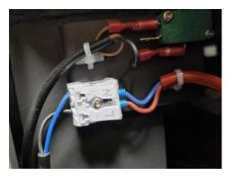
The ceramic ignitor is now installed. Check the function of the ceramic ignitor by starting an ignition and check that the ignitor lights up. If the stove functions as it should, remount the cover plate on the side of the stove.
