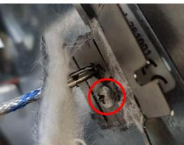
3. Unplug the three connectors from the smoke exhaust fan:
