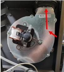
7. Before remounting the sensor, be sure to apply a layer of high temperature resistant silicone to the back of the cover plate. Then reinsert and screw in the screw, insert the sensor and cover with felt:
