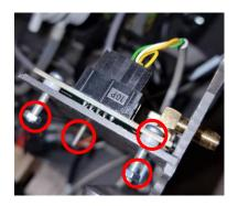
5. Mount the new Wi-Fi module. Please make sure that there are plastic/rubber spacers on all screws so that the module doesn't touch the metal surface.
