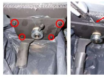
5. Pull out the plate and the auger:
