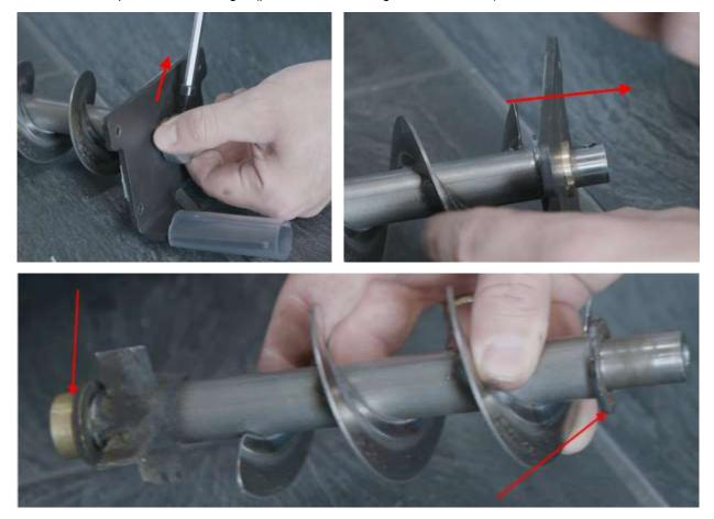
7. Attach the parts to the new auger and reinsert the auger into the stove's pellet tube. Then reattach the plate with the screws:
