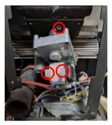
4. Before removing the plate that holds the auger, be sure to place something underneath (e.g., a plastic bag) to catch any remaining pellets. Unscrew the four screws and cut the glue with a knife:
