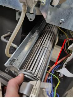
5. Remount the new fan. Make sure to align the holes in the bracket with the fan, and mount the four screws (two on each side):
