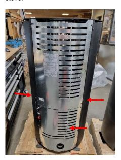
2. Remove the four screws (two on each side), which holds the fan in place:
