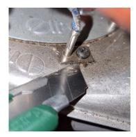
4. Unplug the 4 electrical connectors from the smoke exhaust fan. Remove the fan from the stove, by pulling and twisting the fan, separating it from the internal flue:
