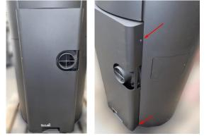
2. Unscrew the 4 screws on the air duct to locate the fan:
