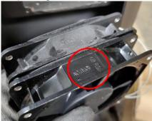
4. Mount the two fans and the air duct with the screws included in the package from the Air Booster:
