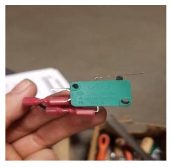
Once installed correctly, this will act as the new door sensor and determine whether the door of the combustion chamber is open or closed. If done correctly no alarms regarding the door should appear.
