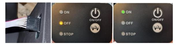
8. If the control panel functions correctly, disconnect the power to the stove and the cable to the control panel. Peel off the sticker covering the glue on the backside of the control panel. Reconnect the cable and place the new control panel where the old one sat.
