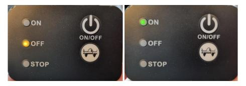
4. If the control panel functions correctly, disconnect the power to the stove, and the cable to the control panel. Peel off the sticker covering the glue on the backside of the control panel. Reconnect the cable and place the control panel where the old one sat.
