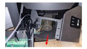
5. Before moving the flat cable, take note of its orientation (see red mark on the cable) to place it the same way on the control board and the new control panel. Replace the cable going from the control board to the control panel with the new cable. The cable needs to be guided behind the motor.
