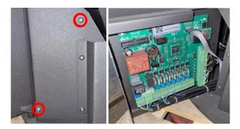
3. Unscrew the 4 screws holding the cover plate (see picture). It might also be necessary to remove some of the cables going to the motor.
