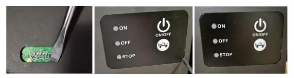
7. Connect the cable to the new control panel. Connect the stove to power and test functionality of both buttons and the LED's.
