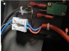
The ceramic ignitor has now been installed. Check the function of the ceramic ignitor by using the hybrid stove with pellets. If the stove functions as it should, remount the cover plate on the side of the stove.
