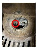
To check if the ceramic ignitor is working, try to turn on the stove without pellets in the auger. When the ignition fails, you can now check if it is warm in the brazier and around the hole to the ignitor. BE CAREFUL, THE IGNITOR AND THE SURROUNDING AREA CAN BE VERY HOT!
