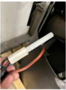
Install the new ignitor in the same spot as the old one. The ignitor is inserted into a small pipe inside the hole. Mount the rubber sealing and press the cable until the igniter is pressing against the top. Then pull the cable 5 mm backwards.
