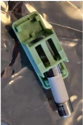
4. Reinsert the fuse holder with the new fuse into the board. Reinsert the control board to the original place.
