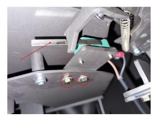
8. Turn on the stove and make sure that the door switch registers the opening and closing of the door. This can be seen in the Aduro Hybrid app or on the stove's display.
