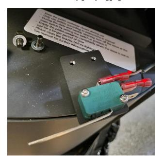
3. Unscrew the two screws to dismount the door switch from the bracket. Remove the old door switch and place the new door switch on the bracket. Screw the two screws back in place:
