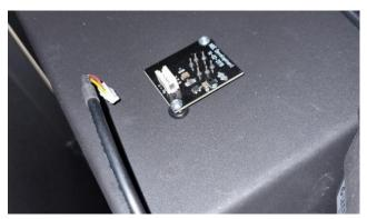
3. Remove the old sensor by unscrewing the two screws holding it in place, then lift it up:
