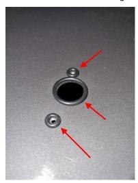
5. Mount the new sensor in the same way as the old one. Please make sure that the holes in the sensor and the sensor itself line up with the holes in the plate. Then screw the screws in place:
