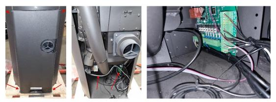
If the stove is placed in a tight space, the control board can also be accessed from the front. Open the lower door of the stove and unscrew the plate on the lower left side of the stove. Gently pull out the board making sure not to damage the board and cables:
