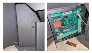
Remove the green connector from the board by tugging on the connector, not the cable. Replace the old sensor by loosening the screws in the connector and replacing the cables:
