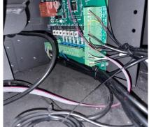
2. If the stove is placed in a tight space, you can access from the front. Open the stove's lower door and unscrew the plate on the lower left side. Gently pull out the board while making sure not to damage the board and cables:
