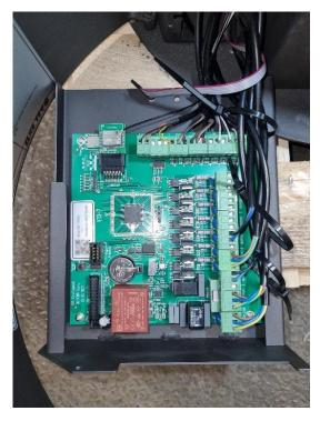
When all cables have been reinserted correctly, test that the stove can turn on again, before tightening the cable ties. Reinsert the board into the stove very gently, while making sure not to damage the board and cables.
