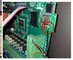
Unscrew the four screws (marked in the picture below), remove the board from the metal plate, and replace it with the new board:
